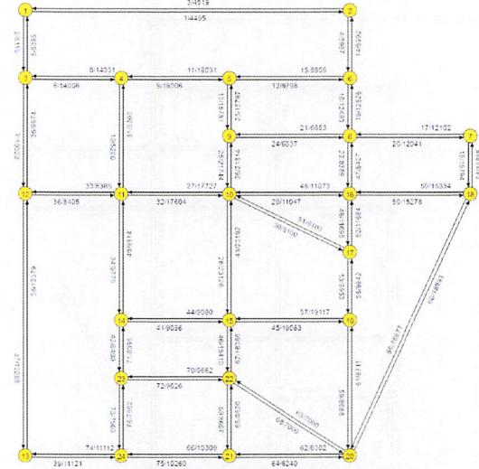
**Fig. 2** Sioux Falls network used in numerical study
